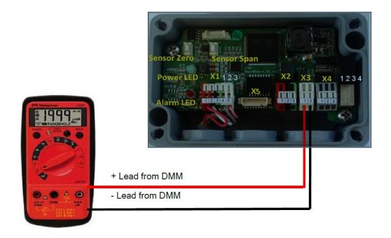
The best way to measure the output signal is to disconnect the unit from the field device and connect a multi-meter across terminals 1&2 on strip X3. Set the multi-meter to measure the correct signal the unit is setup for.
