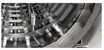
An all-metal hot zone has its place for high-purity process applications that must meet the most stringent demands for part purity, quality and metallurgical accuracy.
