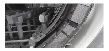
A graphite hot zone is more energy-efficient than an all-metal design, costs considerably less to replace, easier to repair, with longer life.
