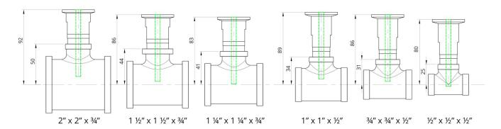
Piping TEE not included. Adapter is KF25 on one end, ½" or ¾" NPT male on the other.
