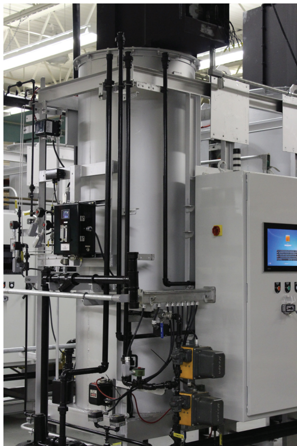
Dew Point AtmoSense™ on Endothermic Gas Generator
