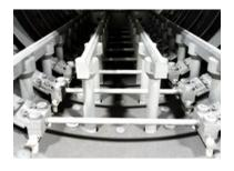
Heavy-duty heating elements and hearth construction for longevity and heavy load capacity
