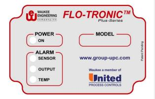
**TEMP** – The TEMP LED indicates when unit electronics (IC) temperature is in excess of 185°F; unit will not function until temperature is below 185°F
