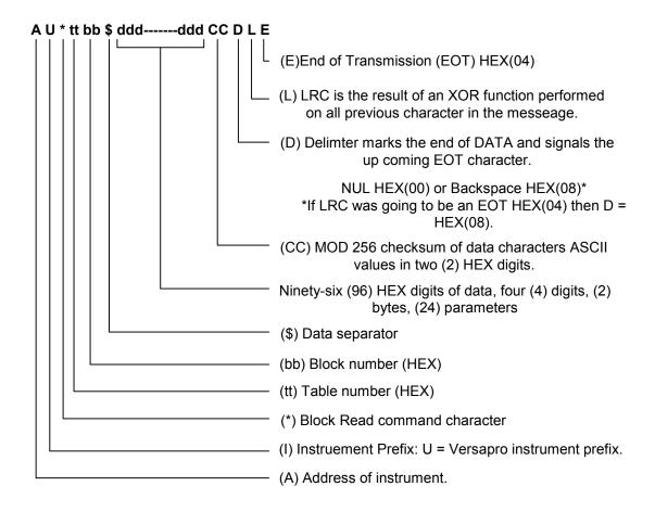
Figure 10 Block Read Response Format
