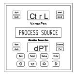
The displayed menu is selected by pressing the ENTER key. The first parameter name in the selected menu list will appear in the center display. The upper LED group continues to display the menu name, and the lower LED group shows the parameter value. A flashing cursor in the lower LED display indicates which digit can change if the parameter value is numeric. The UP or DOWN arrows increase or decrease the digit
