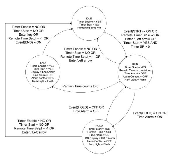
Figure 7 Versapro Timer State Diagram
