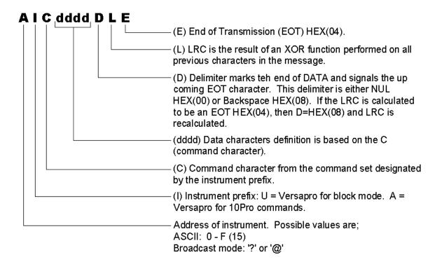
As indicated, the MMI or proprietary mode allows communication using the 10PRO 'A' command protocol or the 'U' block protocol.
