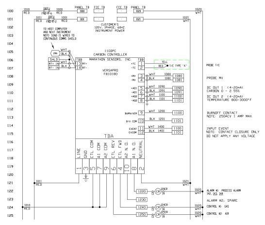
**Figure 2 Typical Wiring Schematic**
