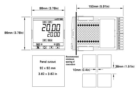
The electronic assembly of the controller plugs into a rigid plastic case, which in turn fits into the standard DIN size panel cut-out shown in Figures 1-3 and 1-4.
