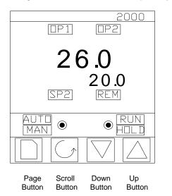
Figure 2-1 Model AACC 2000 front panel layout
