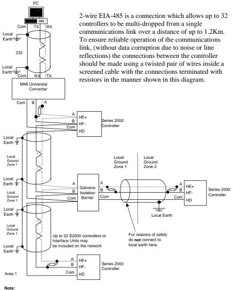
All resistors are 220 ohm 1/4W carbon composition. Local grounds are at equipotential. Where equipotential is not available wire into separate zones using a galvanic isolator. Use a repeater (KD845) for more than 32 units.
