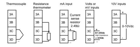
Figure 1-8 Connections for Process Value 2 (PV2)
