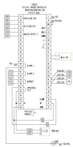
The display below shows a typical wiring diagram for the AACC2000 Carbon Controller:
