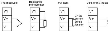
Fig 1-7 Sensor input connections
