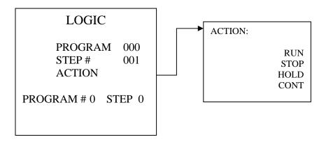
The logic program controls and monitors functions in the instrument that are not normally accessed by the operator. The operator can run / stop / hold / continue any logic program in the instrument. Programs can be started from selected step numbers in the program.
