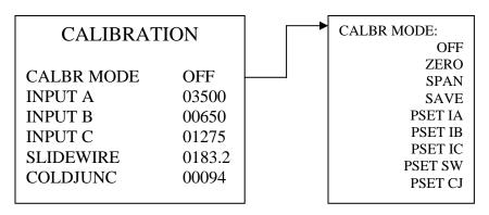
Calbr mode Select the zero or span setting to calibrate either setting on all
