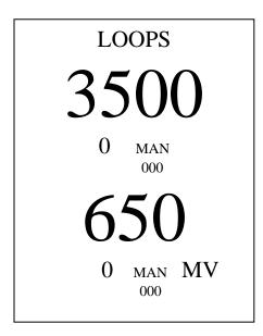
The loops display is an alternate way of display information on the two control loops. The main feature of the loops display is the quad high display of the process variables.
