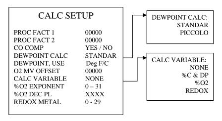
Process factor can be entered to adjust carbon potential calculation.
