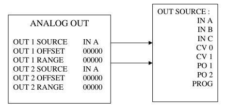
Standard Analog Output Valves are 0 - 5VDC or 0 - 20mA (selectable).
