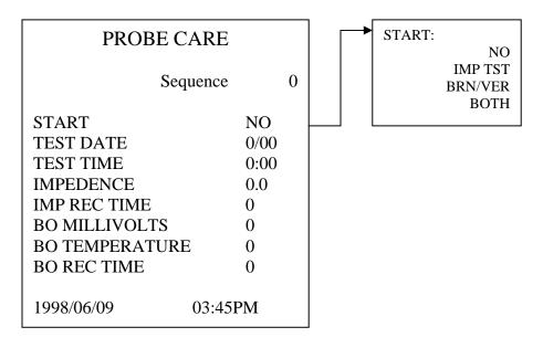
This display shows the latest probe care information from the last maintenance cycle. Impedence is calculated ohms, burn off recovery time is in seconds.
