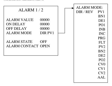
PV - process variable, alarms above this value (Loop 1 or loop 2)
