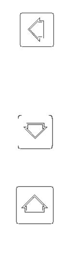
This key is usually used to select which digit is to be modified in a data entry mode. In Manual mode this key will cause the control output to go to the full reverse control direction while the value is displayed in the SET window. In Automatic mode pressing "left arrow" causes the % on-time valve position to be displayed in the SET window. (positive-Output 1, negative-Output 2). In the Programmer Status Display it causes the display to move to a new page.\*\*
