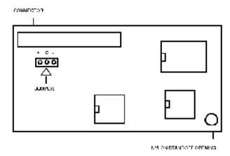
The thermocouple jumper selects either a full upscale or a full down scale reaction to take place when a thermocouple fails or becomes open. The jumper can be found on the thermocouple board, and has two possible settings (see Figure). For full scale upwards, place the jumper from the + to the C, and for full scale downwards, place the jumper from the - to the C.
