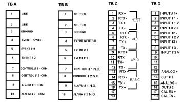
Connections to the unit are made via four terminal blocks, located on the REAR PANEL, labeled TBA, TBB, TBC, and TBD. Positions are numbered from top to bottom. AC power, event, control, and alarm connections are made on TBA and TBB. All communications are located on TBC and all analog I/O signals are located on TBD. Refer to your installation drawings for a complete layout of the electrical connections.
