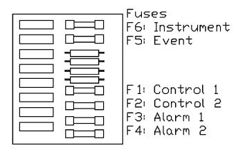
Nearer versions of the Dualpro have only a main fuse for the instrument. Event, Alarms, and Control sources should be fused externally in the control panel.
