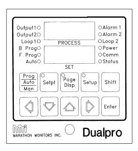
The DUALPRO front panel consists of an upper and lower segment Light Emitting Diode (LED) display, twelve LED indicators, and ten membrane keypads (keys). The upper segmented display shows the process value in normal operation and is referred to as the PROCESS window. When entering parameters, this display will show a message identifying the parameter being entered. The lower display in normal operation will show the process
