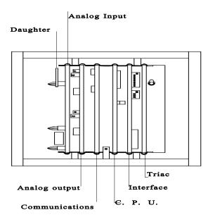
Remove the board that may be causing the problem and exchange it for a new one. **Note : If removing or**
