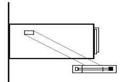
3. Repeat step 2 for the opposite side of the unit.4. With a 7/16" socket or wrench, alternately tighten bolts on either side of the instrument until the springs are compressed halfway to ensure rigidity of mounting.
