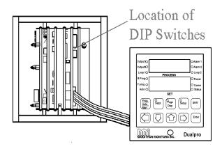
counter-clockwise direction. Carefully remove the FRONT PANEL, but DO NOT remove the ribbon cable connecting the FRONT PANEL to the INTERFACE BOARD. Safely support the FRONT PANEL near the instrument. Adjust DIP switches for the desired operating mode. When switch adjustments are complete, replace FRONT PANEL to prevent contamination.
