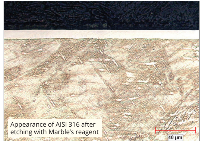
Appearance of AISI 316 after etching with Marble's reagent NANO-S™ also improves the corrosion resistance of the layer produced resulting in a surface capable of resisting a chemical etching better than the base material.
