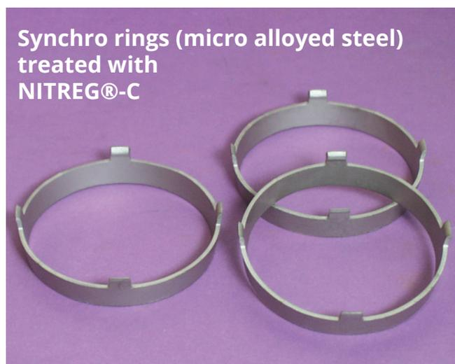
Whenever your nitriding specification calls for a higher  $\epsilon$  content, **NITREG®-C** is the sure answer. Synchro cones, shown in the adjacent photograph, manufactured from a low carbon micro alloyed steel, constitute an application where the major requirement was to have more than 80% of the  $\epsilon$ -phase present in the white layer. Results of X-ray diffraction tests showed the  $\epsilon$  content to be 97-98%.
