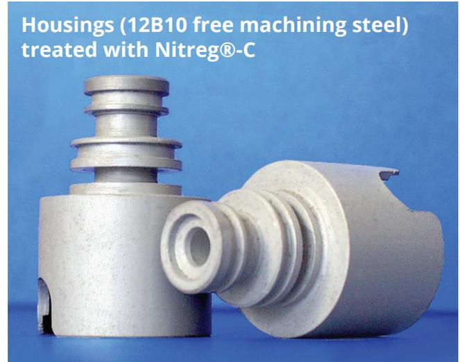
For those applications where high  $\epsilon$ -content, excellent wear resistance and enhanced corrosion resistance are simultaneously required, a combination of **NITREG®-C** and post-oxidation as in **ONC®** is the winning solution.
