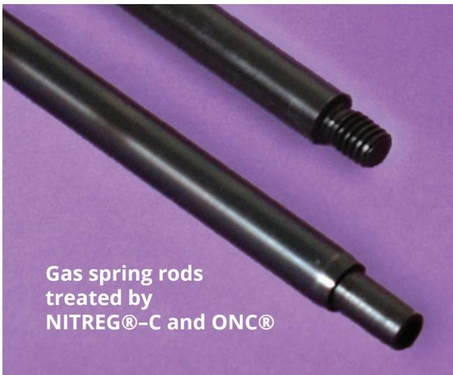
Specifications for gas spring rods made of 1040 steel required a surface hardness of over 400 HV and a corrosion resistance measured by a minimum of 144 hours in salt-spray per ASTM B117.
